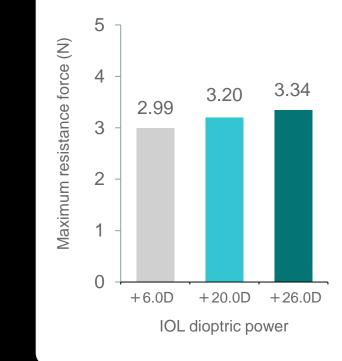
[Method] Resistance forces were measured by Table-top Material Tester EZ-S (Shimadzu) when the plunger was depressed at 15mm/min. (n=1 per dioptre)
