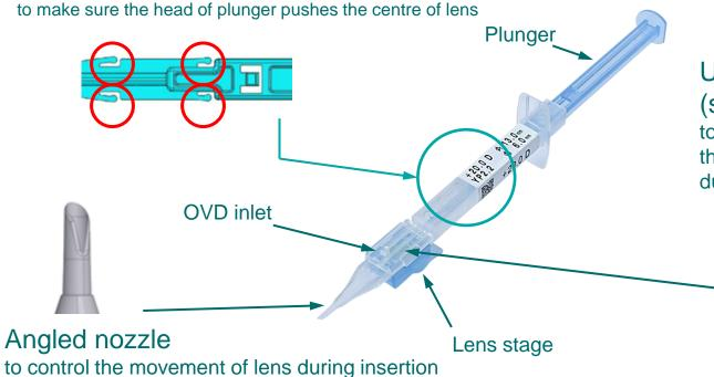
Unique plunger (scoop-shaped plunger) to control the attitude and the movement of lens during insertion
