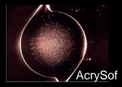
• With 20 AcrySof SA60AT IOLs extensive measurements with the same experimental procedure were performed. Here, the formation and development of severe glistening could be observed. The glistening start to appear between 5-24 hours at 45°C. Their number increases over time up to 60 days. After 60 days a plateau could be observed where the IOL optic area appeared saturated with the microvacuoles.
